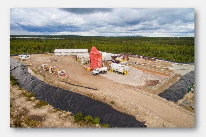
Surface Access Borehole Resource Extraction – or "SABRE" for short – is a proprietary mining method designed to excavate underground material from surface using a water jetting process
