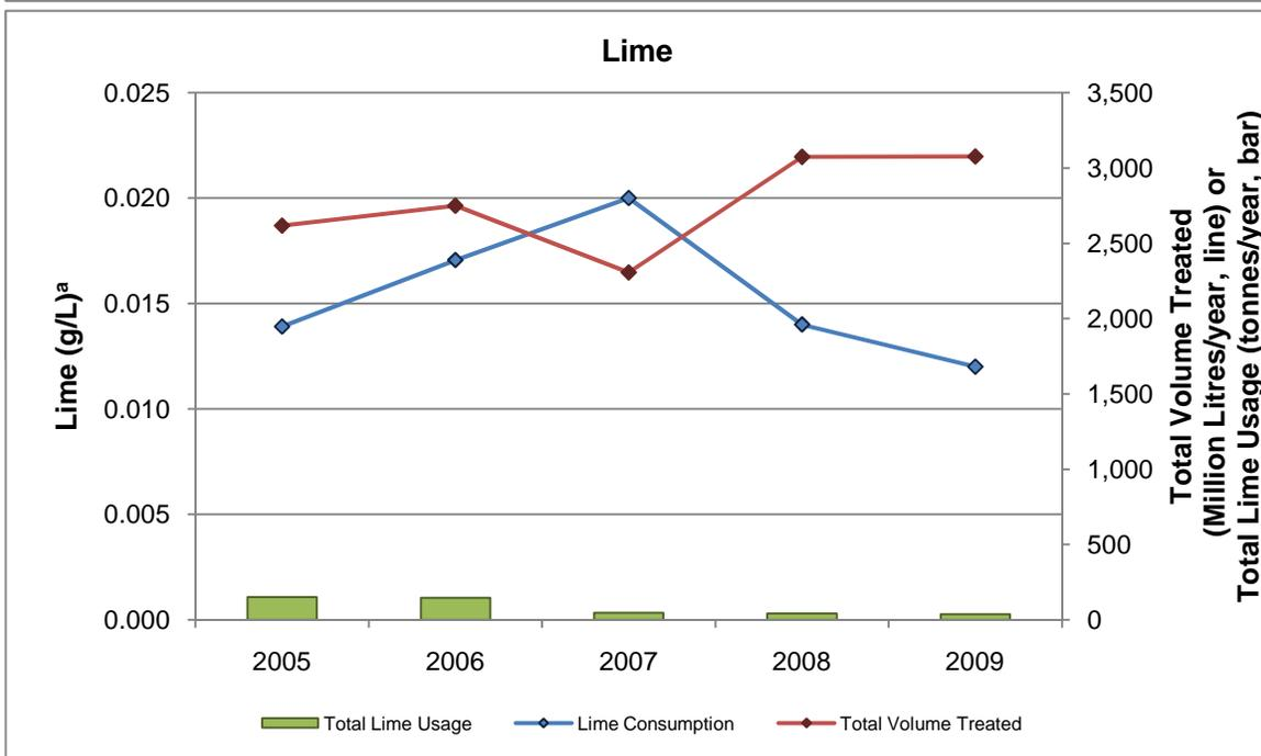
**Figure 3.13: Comparison of total reagent consumed versus total volume treated at Quirke TMA from 2005-2009. <sup>a</sup> including in situ cell lime additions.**
