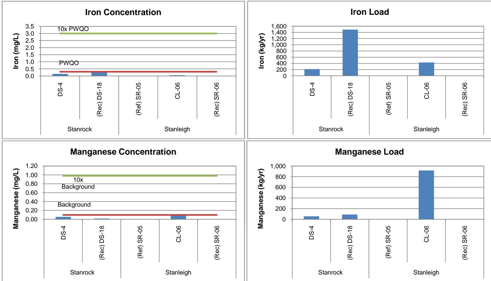
**Figure 4.6: Mean concentrations and loads at monitoring stations downstream of Stanrock and Stanleigh TMAs, 2005-2009, (Rec) denotes receiving environment station, (Ref) denotes reference station. Iron and manganese not measured at SR-05 and SR-06.**
