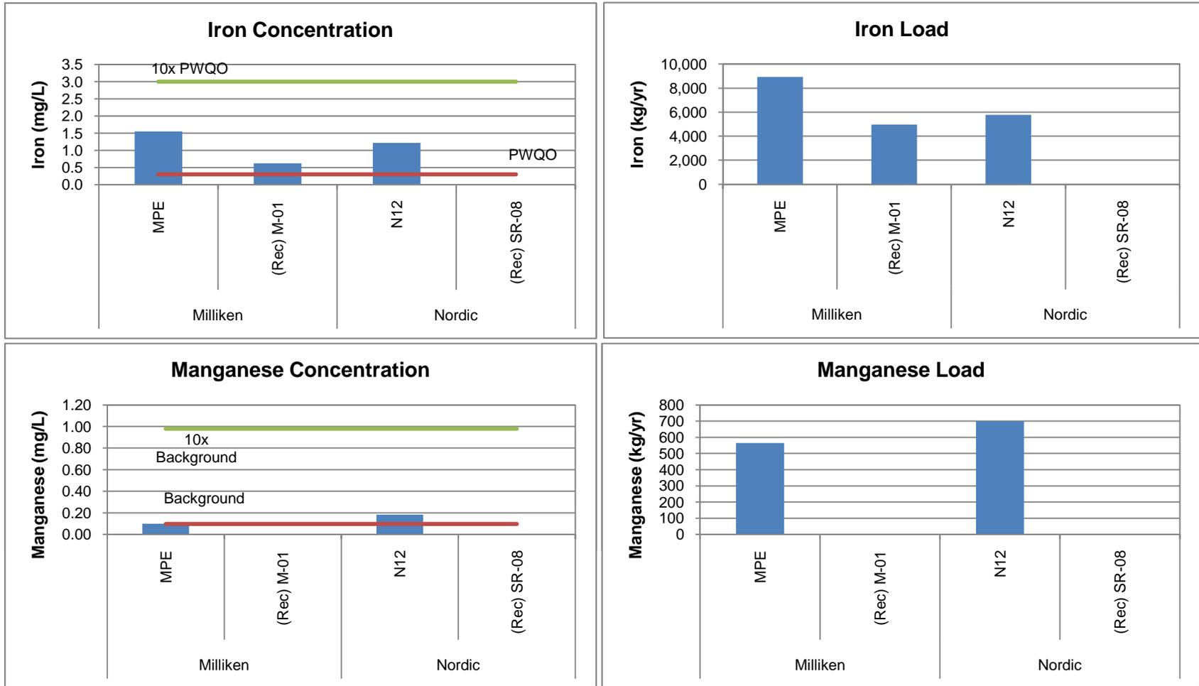
**Figure 4.8: Mean concentrations and loads at monitoring stations downstream of Milliken and Nordic TMAs, 2005-2009, (Rec) denotes receiving environment station. Iron not measured at SR-08 and manganese not measured at M-01 and SR-08.**
