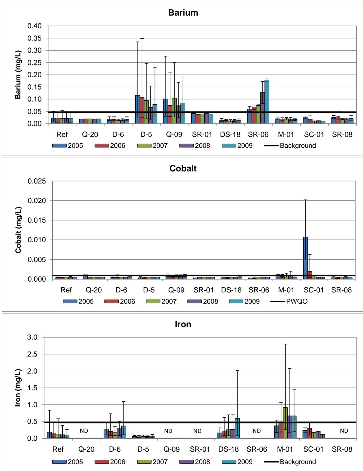
**Figure 5.1: Mean, minimum and maximum water concentrations over time at mine exposed stations relative to pooled reference stations and water quality benchmarks. ND denotes no data available for that station.**
