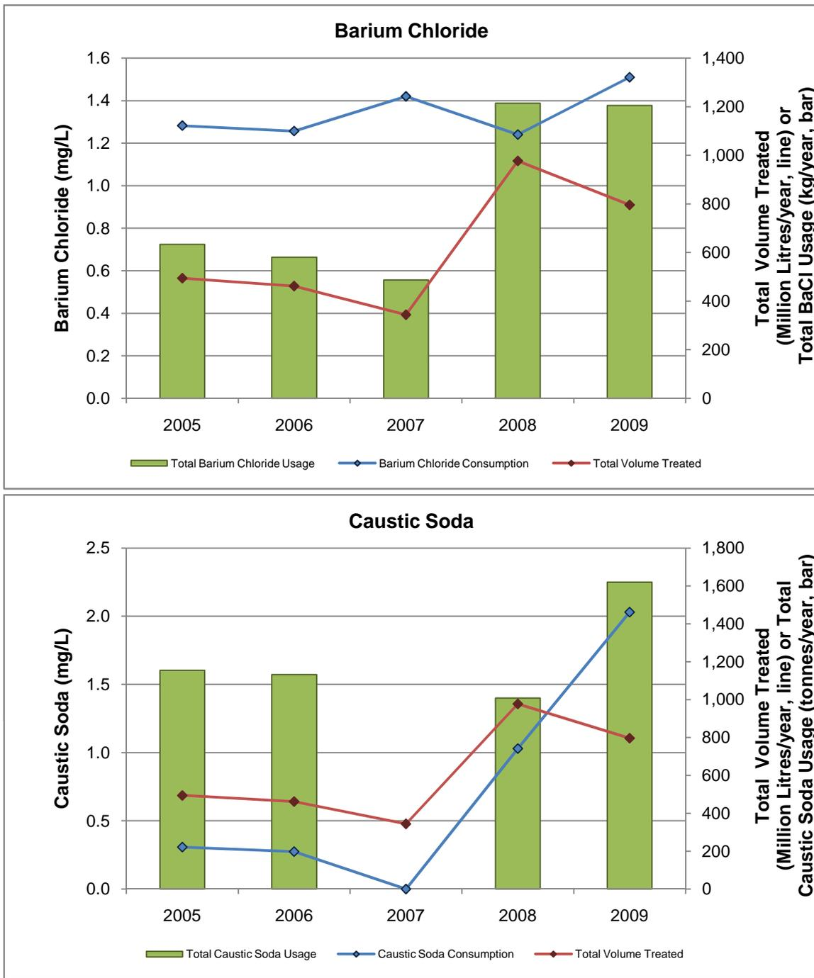
**Figure 3.4: Comparison of total reagent consumed versus total volume treated at Denison TMA-1 from 2005-2009.**
