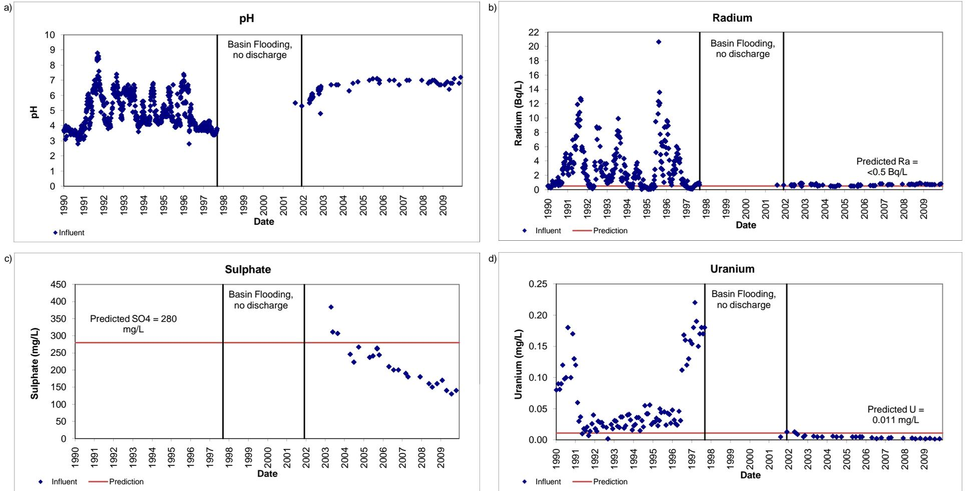
Figure 3.26: Water quality at the Stanleigh TMA ETP influent (CL-04) relative to predictions for 10 years (2012) post-decommissioning.
