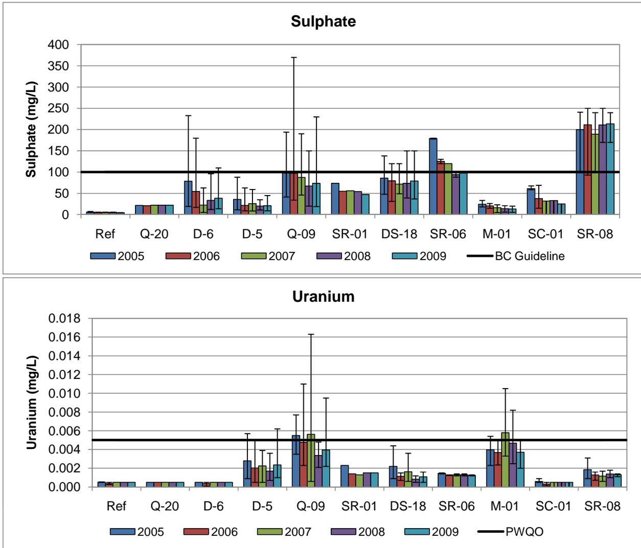
**Figure 5.1: Mean, minimum and maximum water concentrations over time at mine exposed stations relative to pooled reference stations and water quality benchmarks. ND denotes no data available for that station.**
