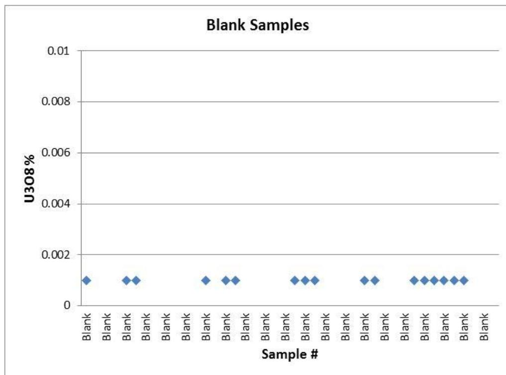
Figure 11-11: Results of the 2013 blank reference samples for  $U_3O_8$ , Tthe Heldeth Túé.
