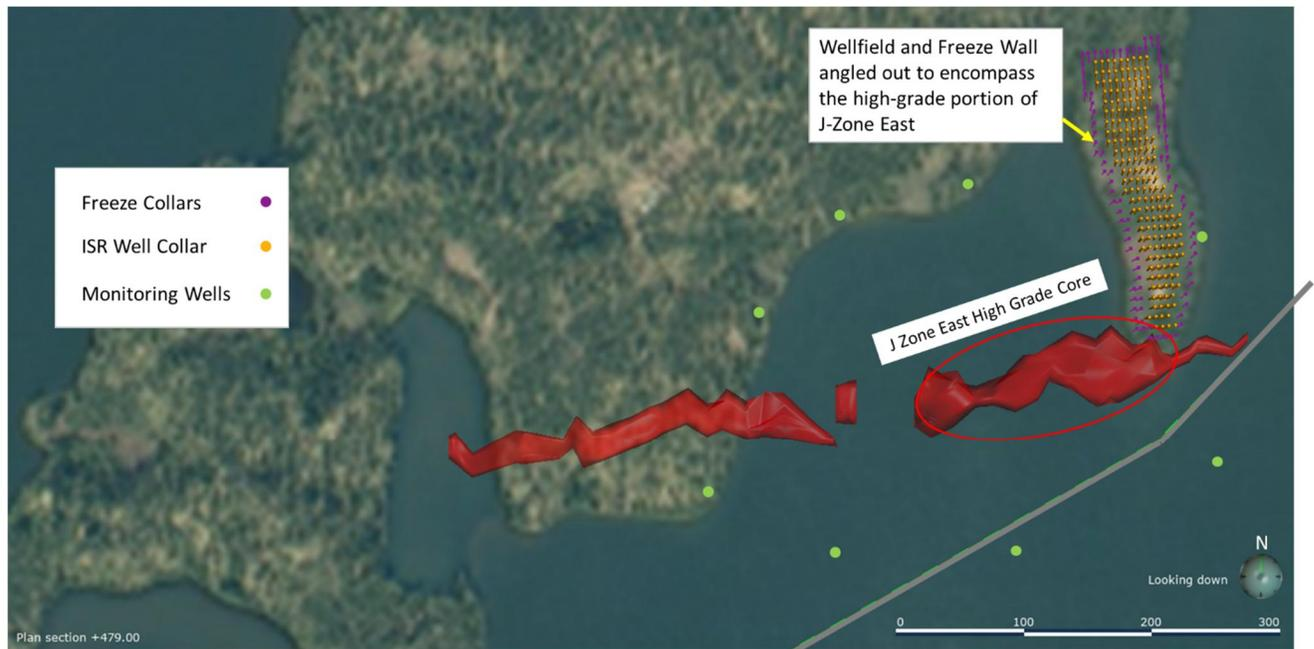
**Figure 16-3: Tthe Heldeth T   (J Zone) Wellfield and Freeze Wall Plan View at Surface.**
