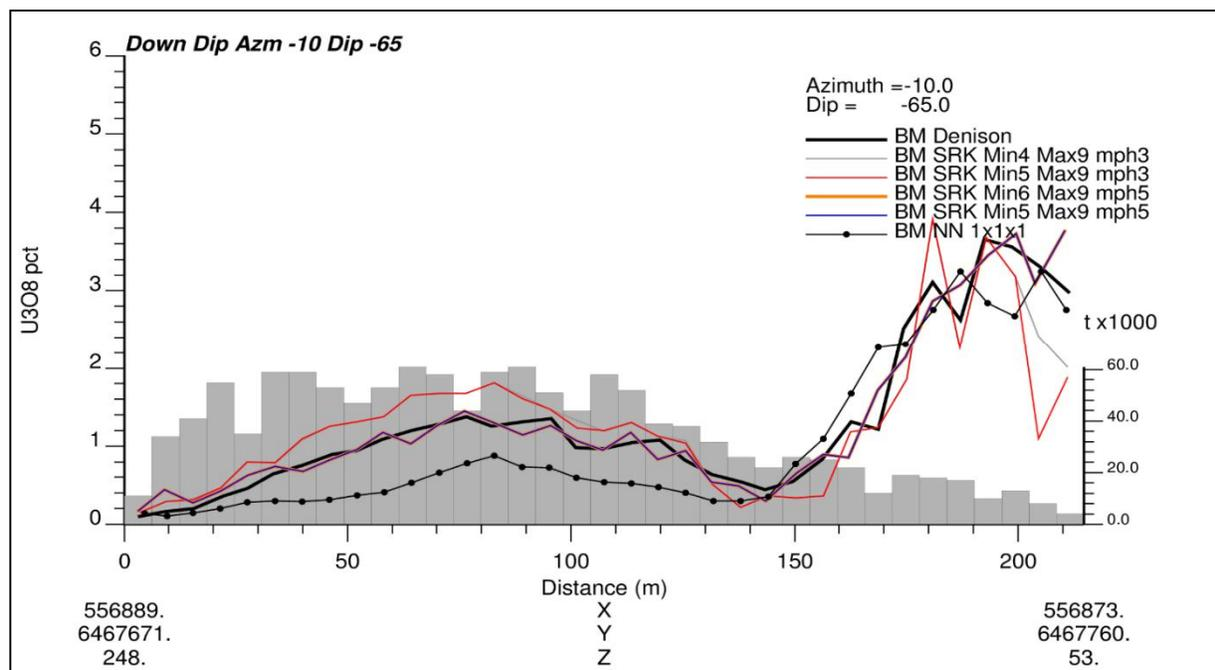
**Figure 14-9: Swathplot Comparing  $U_3O_8$  Grades from Estimated Models for Huskie lens 2, Oriented Down Dip. Histogram represents model tonnage.**
