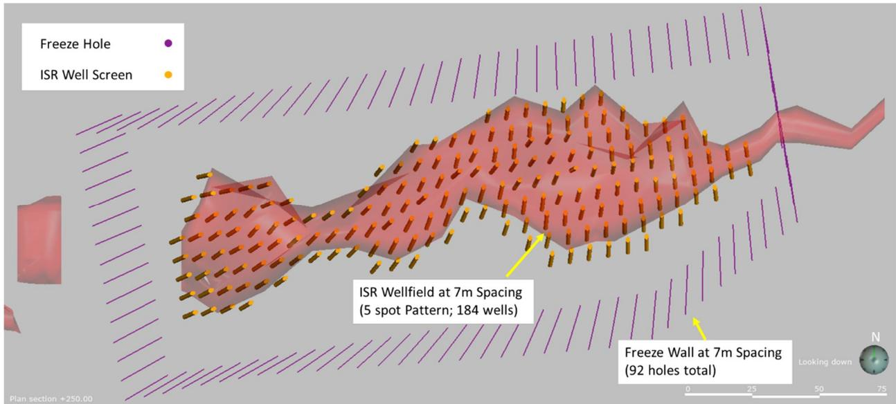
**Figure 16-4: Plan View of Tthe Heldeth T   Freeze Wall and ISR Wells at Ore Level.**
