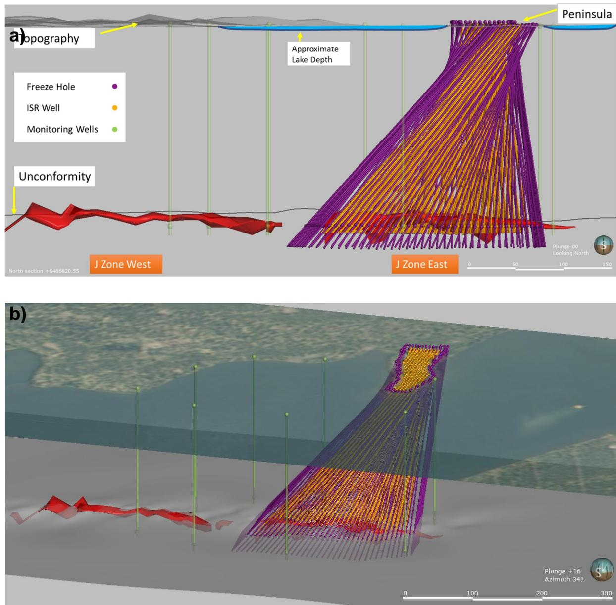
**Figure 16-7: Conceptual 3D ISR Mine Model of Tthe Heldeth Túé. Views include: (a) long section looking north, (b) oblique view looking northwest.**
