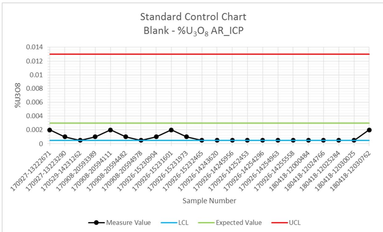
Figure 11-19: Analytical Results for Blank Control Sample for Huskie.
