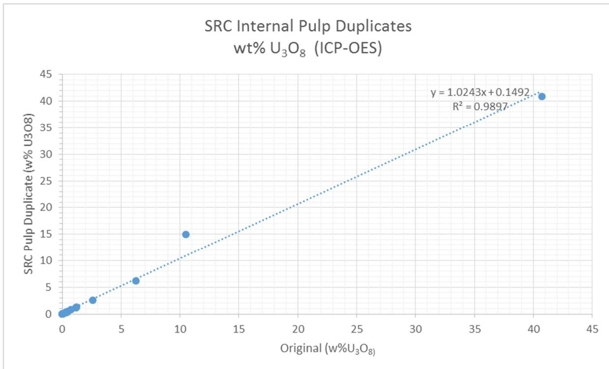
**Figure 11-20: Analytical Results for the Pulp Duplicates Versus the Original Assay Samples for Huskie.**
