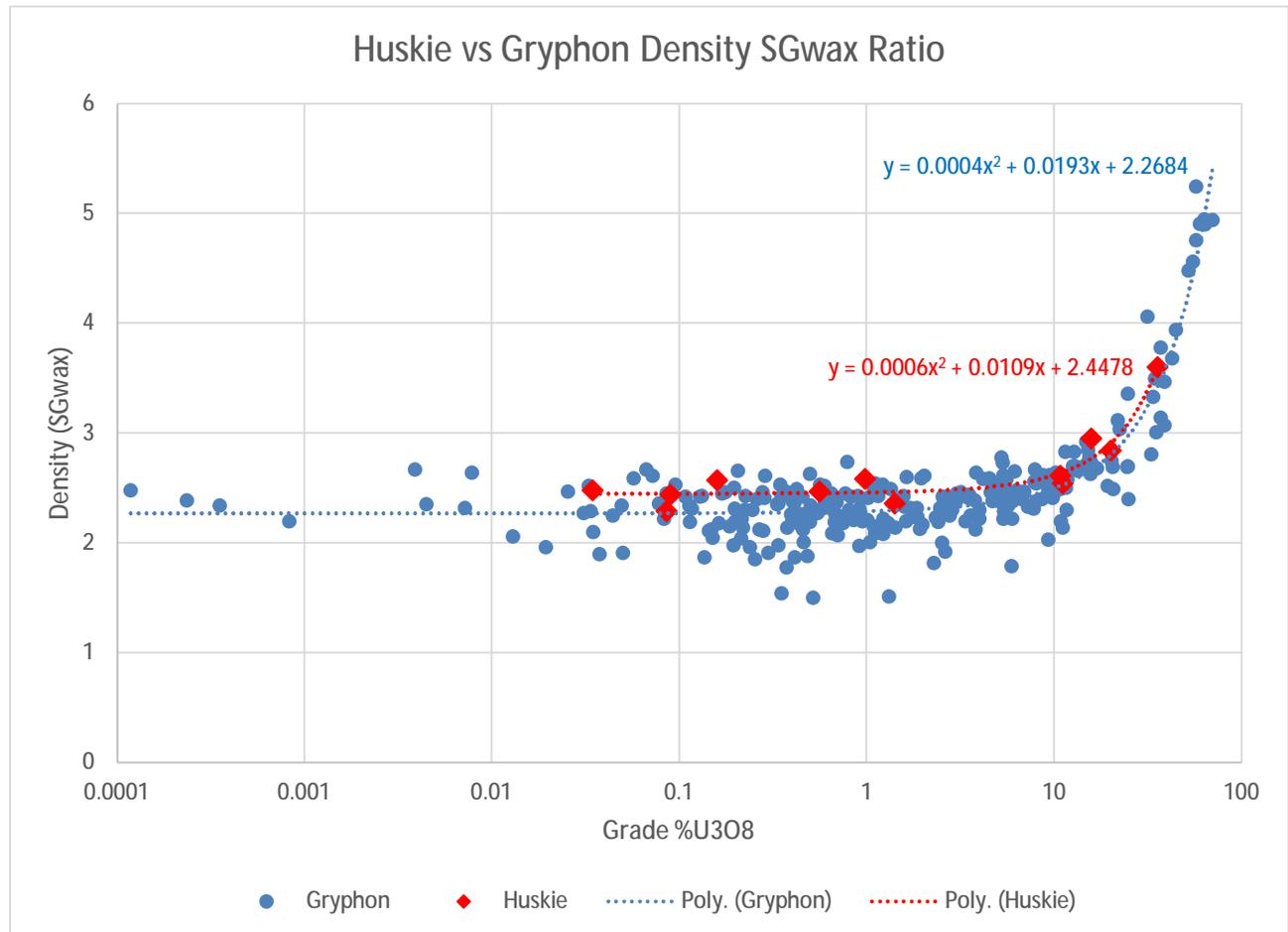
**Figure 14-6: Gryphon and Huskie Deposits Grade (%U<sub>3</sub>O<sub>8</sub>) and Density (SGwax – g/cm<sup>3</sup>) Regression Curves.**
