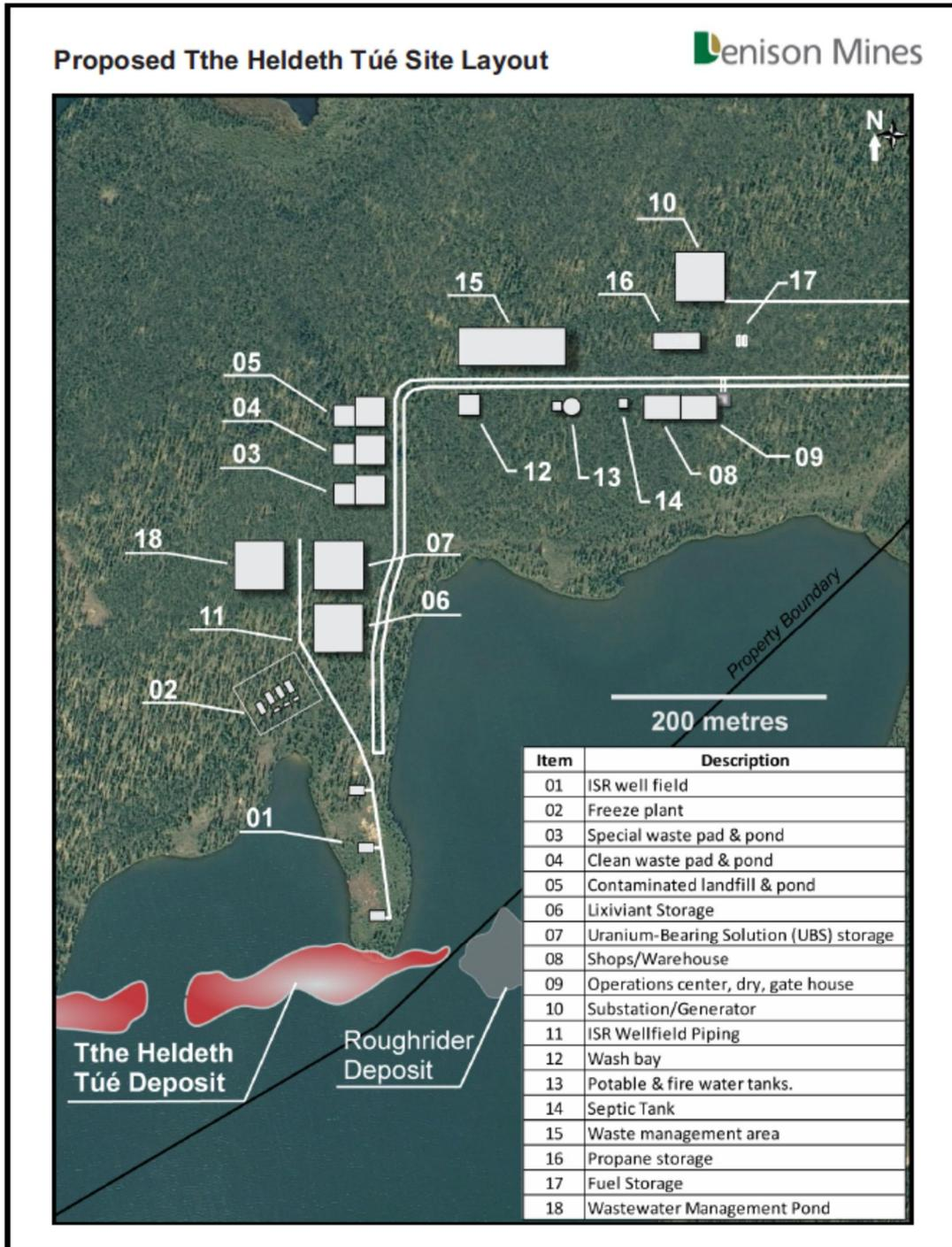
**Figure 16-6: Tthe Heldeth Túé (J Zone) Plan View Showing Wellfield, Header Houses, and Well Lines.**
