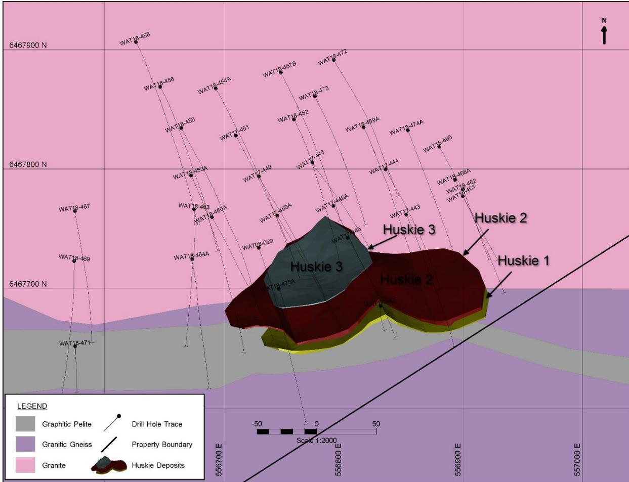
**Figure 7-7: Geology Plan Map Showing Drill Hole Traces and the Huskie Deposit Mineralized Wireframes.**
