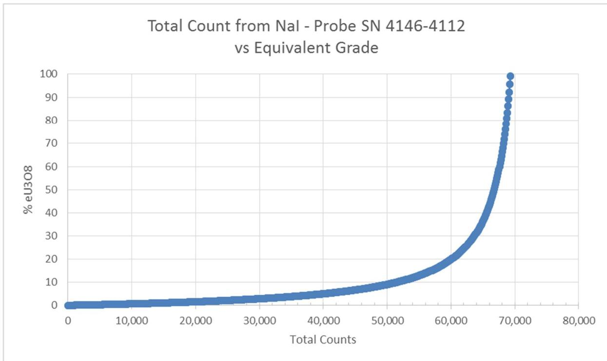
**Figure 10-1: Calibration curve for the NaI scintillation crystal in Mount Sopris probe SN 4146-4112.**
