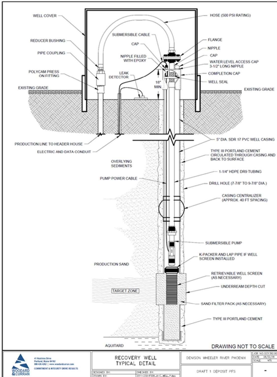
Figure 16-5: Typical Recovery Well Design.
