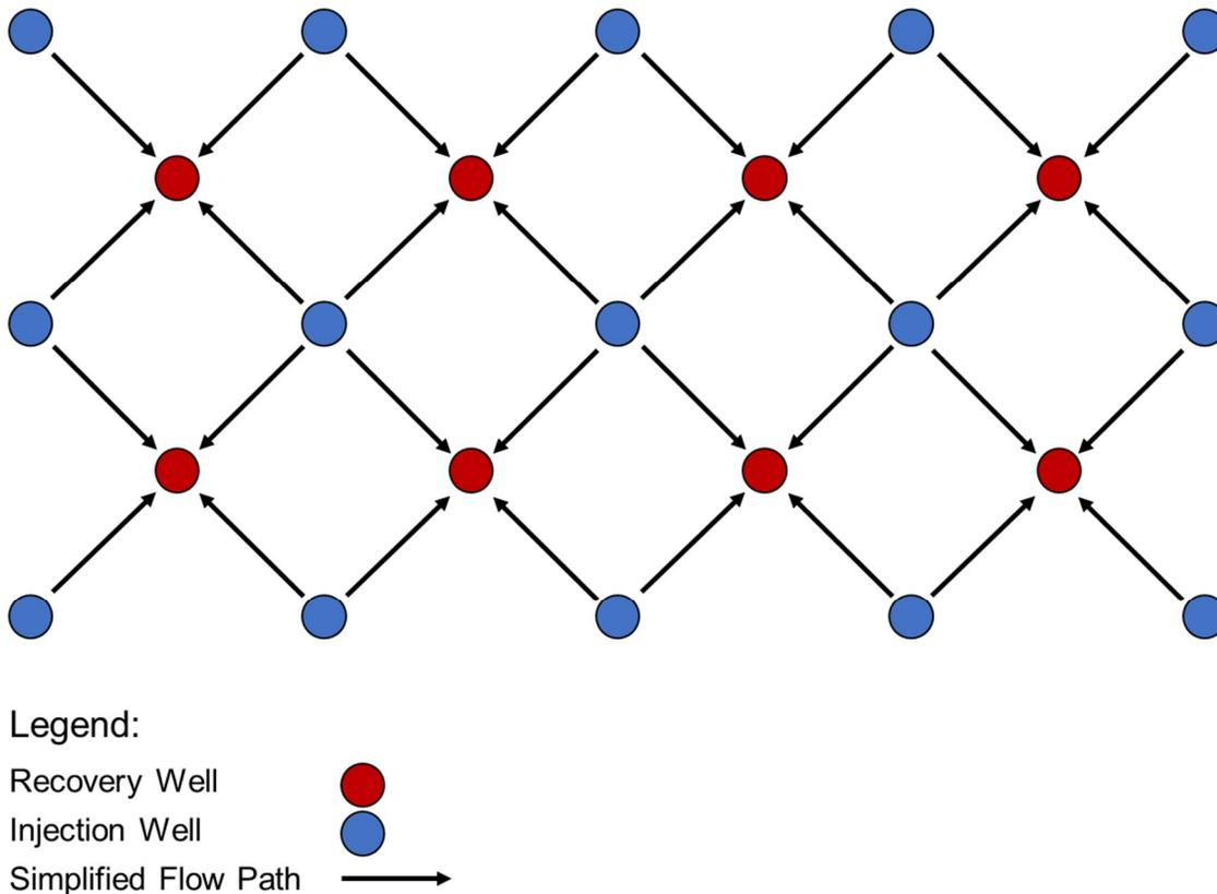
**Figure 16-2: Conceptual 5-Spot ISR Wellfield Design.**
