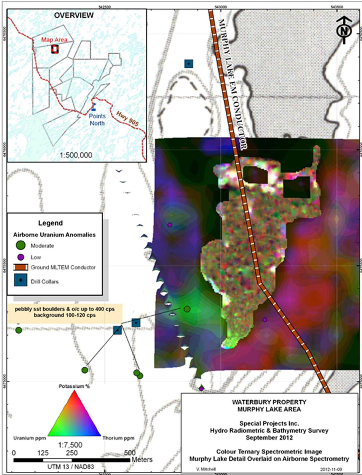
Figure 9-5: Murphy Lake hydro-radiometric survey area and contoured lake bottom radiometric results (from Fission Energy Corp, 2012).
