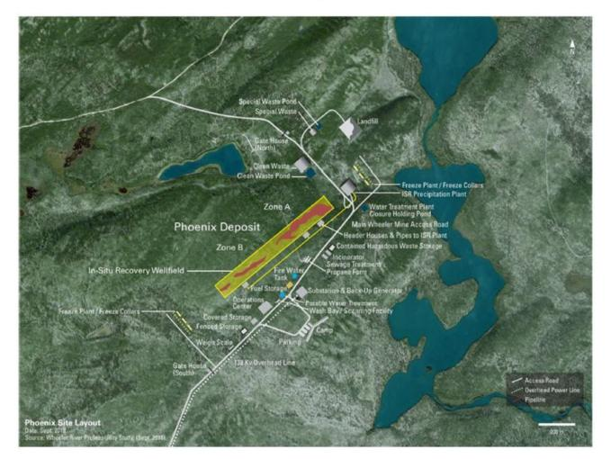
The figure above reflects the 2018 PFS' conceptual plan for the Phoenix operation's surface facilities, showing the relative scale and nominal footprint of site infrastructure, including (all estimated sizes are approximate):
