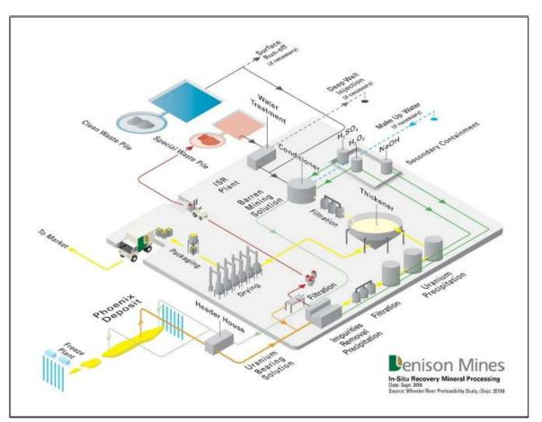
Broadly, the 2018 PFS ISR processing plant design for Phoenix involves the beneficiation of the uranium bearing solution recovered from the wellfields and pumped to the processing plant, as described below:
