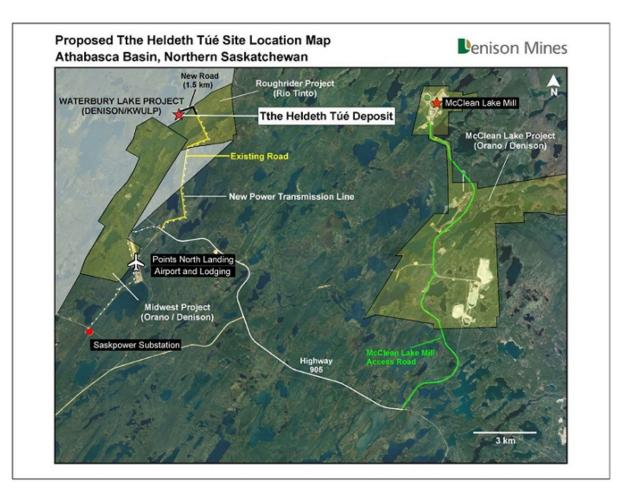
Due to the initial capital costs required to install a standalone processing plant at THT, processing of the THT deposit is expected to occur at the McClean Lake mill with the UBS being transported via trucks from the THT site to McClean Lake on the existing provincial road (45 kilometre one way). The trucks would complete the return trip to THT loaded with lixiviant.
