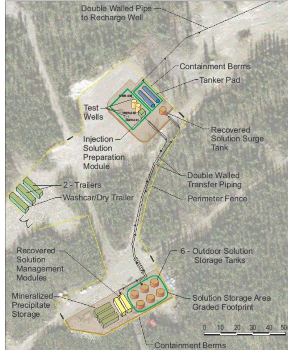
**The Phoenix FFT** was designed to validate and inform various feasibility study elements for use of **In-Situ Recovery (ISR)** mining, including production and remediation profiles, and is planned to occur in three phases. The first phase commenced in **H2'2022**:
